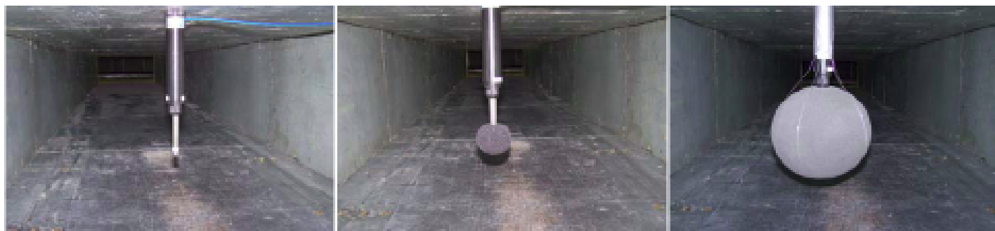
Figure 1: Test set-up in anechoic room showing unprotected microphone and fitted with manufacturer's standard 60mm test and ACO Pacific model WS-07
